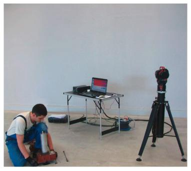
Each BW-Fixator® will be set individually into the reference coordinate system. Thus, there are no subsequent errors. 每个BWF固定器将逐一在确定的参考坐标系中被校准。不会出现累积错误。
