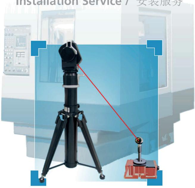
Pre-installation of BW-Fixators® with laser tracker.
