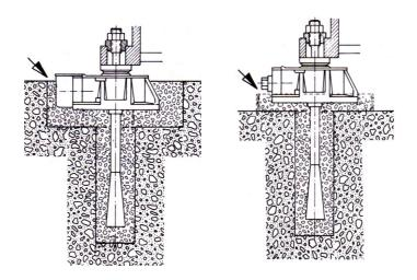
Remove the centering sleeves, makeshift wedges and grouting frames when the grouting has set. Replace the centering sleeve by a variety "p" set (spherical washer and pan).
