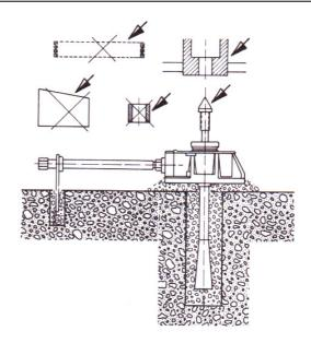
When the machine is down in place, remove the bolt end caps, install a variety "p" set (spherical washer and pan) and the anchor bolt nuts.
