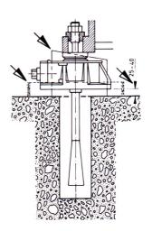
No frames will be required for grouting flush with the foundations, but the dimension "z" (listed in the catalogue and depending upon the BW-FIXATOR size) must be adhered to.
