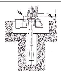
Grout the anchor bolts and BW-FIXATORS flush with or on top of the foundations.
