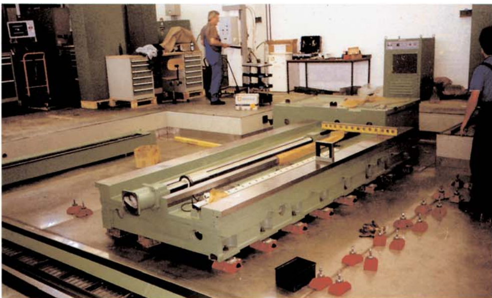
Completed group of BW-Fixators with machine bed installed
