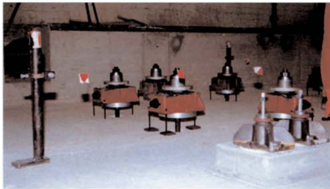
Each BW-Fixator is positioned by measuring back to the same reference axis which eliminates measurement errors
